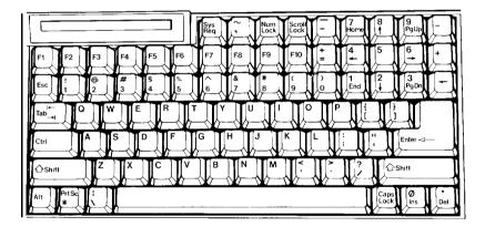
Certain keys on your keyboard serve special functions when your computer is running application programs. For instructions on how to use keys for specific software functions, consult the manual that came with the program you're running. The Num Lock, Scroll Lock, and Caps Lock keys work as toggles; press them once to turn on a function and again to turn it off. When a function is on, the corresponding light on the status indicator bar is illuminated. When a function is off, the light is off.
